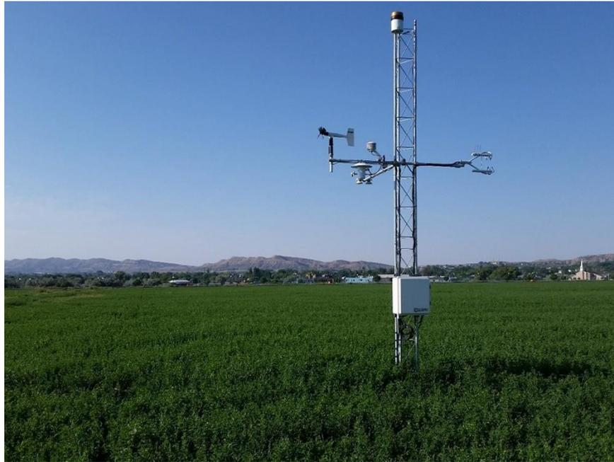
**Figure 2. Eddy Covariance Tower located over an alfalfa field near Vernal, Utah**
